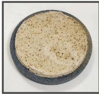
Figure 2- Drilling Mud standard filter-cake on 50-micron disc.
