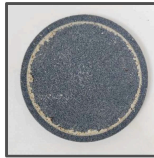
Figure 3- Mud cake after cleanup with Petrolize® Enzyme solution @ 100°C in 8 hours
